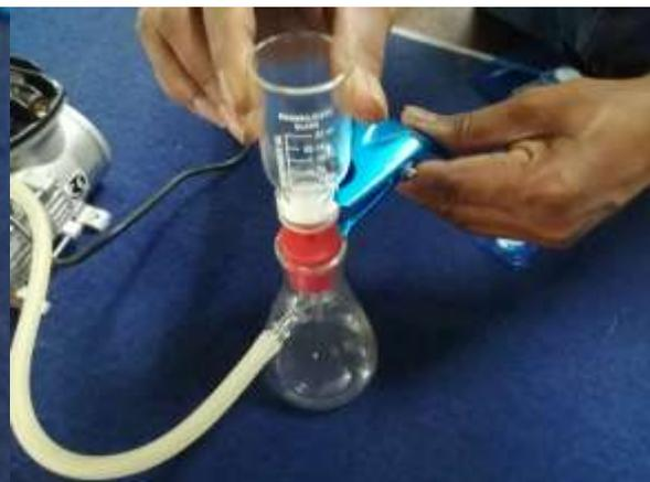
**Secure the assly with the tongs**
