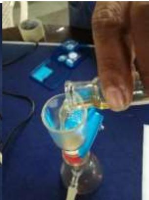
Pour oil in the cylinder and let it drain in the flask.
